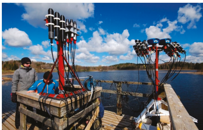
Figure 4. All the radiance and irradiance radiometers were mounted in common frames during the LCE-2 outdoor experiment. Left frame—irradiance sensors; right frame—radiance sensors.
