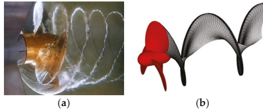
Figure 8. The wake surface model of a propeller: (a) experimental results [38], (b) numerical model.
