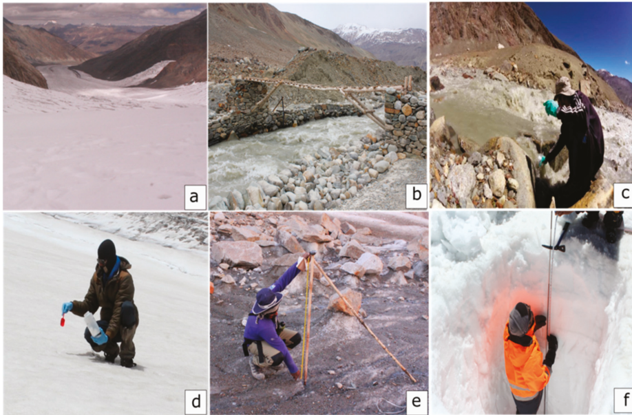
Figure 2. Fieldwork on the Sutri Dhaka Glacier and catchment: (a) Downstream synoptic view of the Sutri Dhaka Glacier showing the accumulation and ablation zone; (b) hydrological observation site; (c) meltwater sampling; (d) snowpack sampling; (e) stakes coordination and measurements; (f) snow pit excavation and density measurements.
