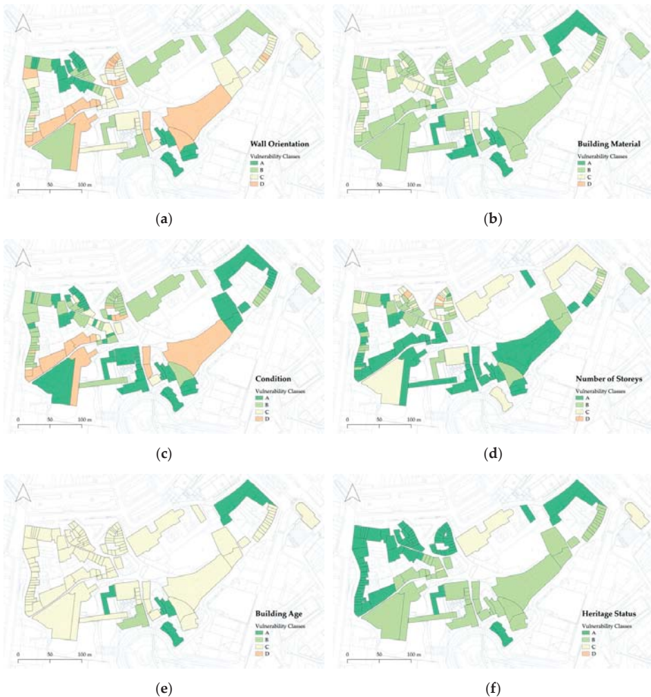
Figure 7. Mapping of the spatial distribution of the vulnerability classes: (a) Wall Orientation; (b) Building Material; (c) Condition (or conservation status); (d) Number of Storeys; (e) Building Age; (f) Heritage Status.
