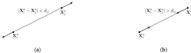
Figure 5. Two possible forces at nodes X_i^n and X_j^n : (a) repulsive force and (b) attractive force.
