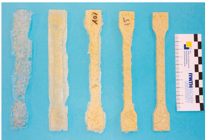
Figure 9. The Cg1-1 series containing an increasing amount of shredded feathers cured in dog-bone shaped moulds. From left to right: 0 (Cg1-1), 5, 10, 15, and 20 wt-% (Cg1-1F).
