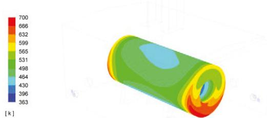
**Figure 7.** Temperature of the load surface after 2 h of the heat treatment—case 7.
