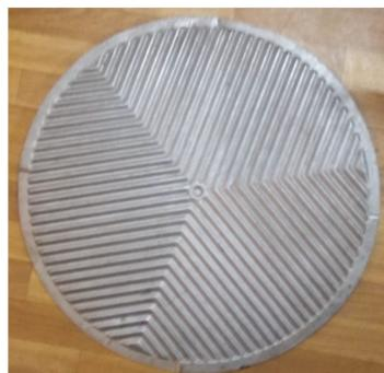
**Figure 1.** The plate of WPHE for an ammonia synthesis column.
