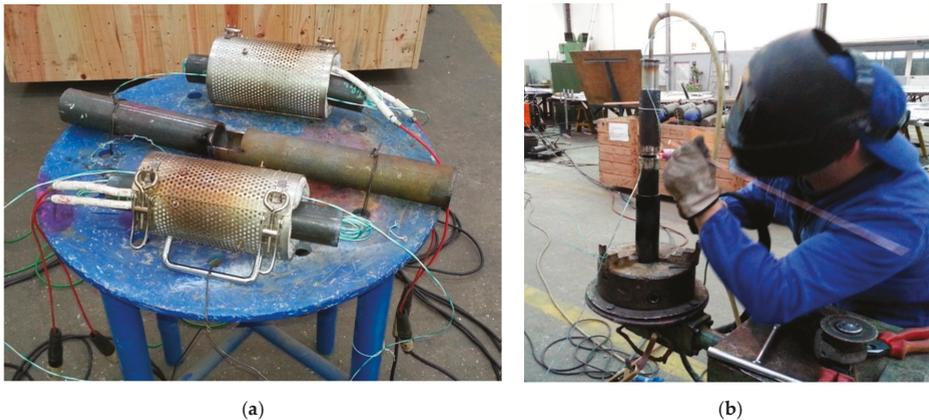
**Figure 2.** (a) Pipes preheating setup and (b) Pipe welding.
