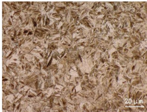
**Figure 1.** Optical microstructure of the hot-stamped hardened steel.
