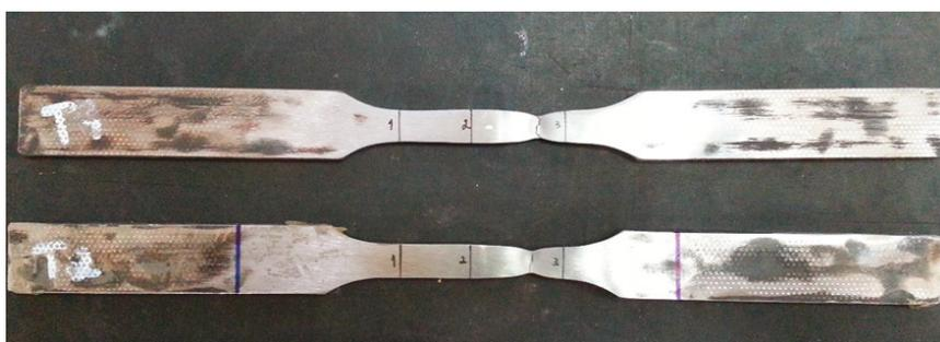
Figure 8. Aspect of the samples used in tensile tests after rupture. Line 2 indicates the welding zone.
