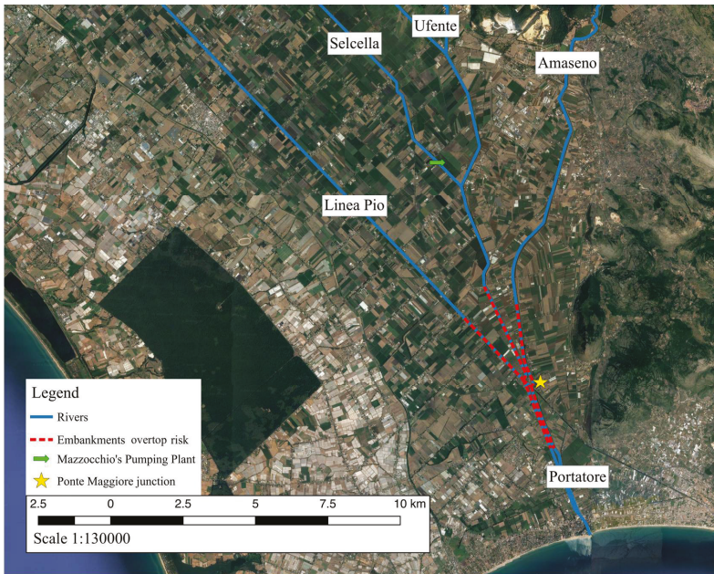
Figure 13. High risk of embankment overtop near Ponte Maggiore's junction using a 100-year return period hyetograph as the boundary condition for the hydraulic simulation.
