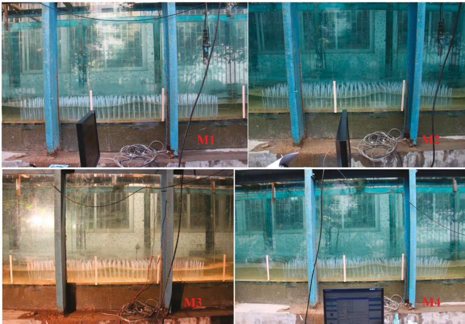
Figure 2. The picture of four materials of the flexible rods bending during the experiment.
