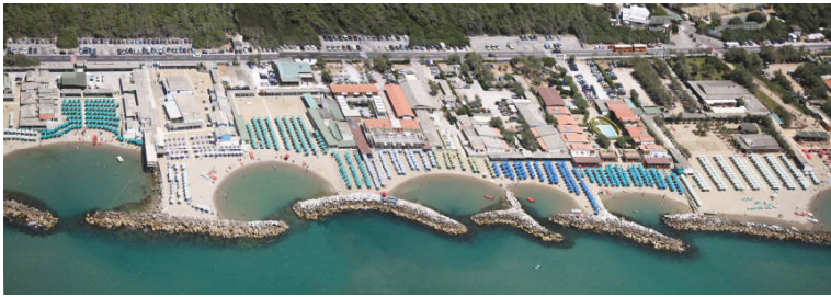
Figure 15. Between Marina di Pisa and Tirrenia: coastal armouring following emergency, un-coordinated interventions (Photo Provincia di Livorno).
