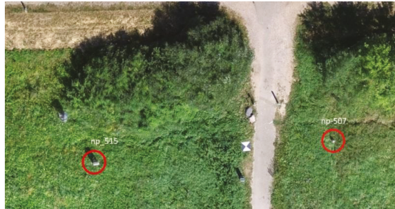
Figure 4. Examples of identified objects. The red circles define the small objects location, whose measured coordinates are used to adjust the 3D model.
