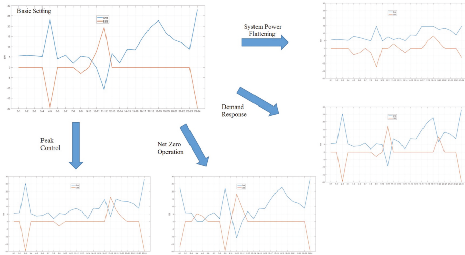
Figure 2. Diagram showing the changes in system power usages, ESS charging/discharging according to the external operating conditions.
