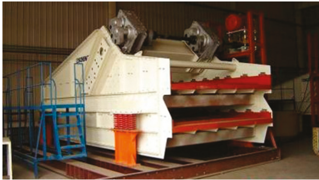
Figure 1. The SLK3661W double-deck linear mining vibrating screen, unloading side view.
