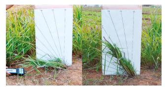
Figure 2. Push-pull gauge used to measure the culm strength in the mutant population.
