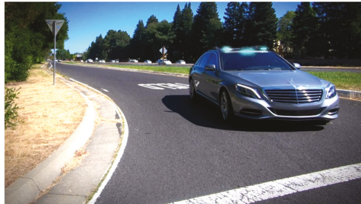
Figure 2. The study compared three eHMI test conditions within a driverless self-driving vehicle (SDV). This figure shows the status+intent eHMI (test condition 3). Two steady lights at the fake sensors indicate the automated status; a slowly flashing light at the windshield indicates its intent to yield to the pedestrian. For the status eHMI (test condition 2), the two steady lights were engaged. Without an eHMI (test condition 1), no lights were engaged. Reproduced with permission from Faas, Kao and Baumann, A longitudinal video study on communicating status and intent for self-driving vehicle–pedestrian interaction, Proceedings of the SIGCHI Conference on Human Factors in Computing Systems (CHI '20) ; published by ACM, 2020, doi: 10.1145/3313831.3376484.
