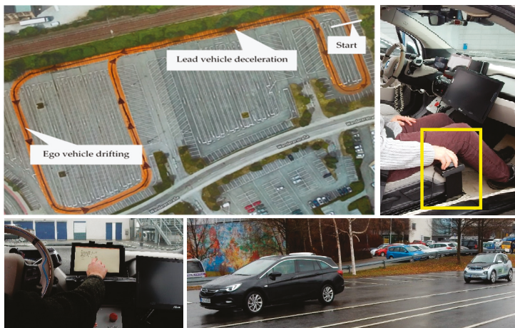
Figure 1. Test track depicting the two take-over situation locations (top row, left), the execution of lateral vehicle control via Wizard-of-Oz (top row, right), experimental setup within the ego vehicle (bottom row, left), and the two vehicles involved in the driving scenario (bottom row, right).
