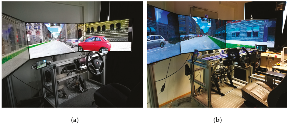
Figure 6. Modular driving simulators. (a) Manual vehicle setup; (b) Automated vehicle setup with blue LED-strip.
