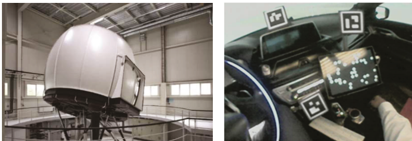
Figure 1. Dynamic driving simulator from the outside (left) and mockup interior with the Surrogate Reference Task (SuRT) tablet used in the current study (right).
