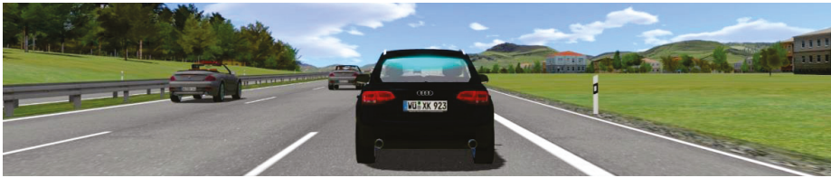
Figure 1. Marked automated vehicle with a cyan LED strip in the upper part of the rear window in the driving simulation.
