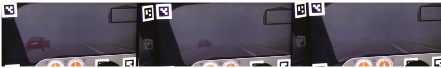
Figure 5. Visibility in the foggy scenarios. Vehicles disappear at a distance of approximately 33 m.
