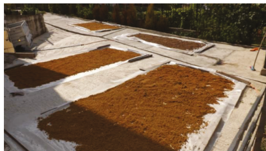
Figure 5. The drying of the vegetal material at a temperature of about 25–27 °C after the treatment with a sodium silicate solution.
