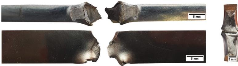
Figure 8. Fractured sample after separation by joining the hinges (three views of the same sample).
