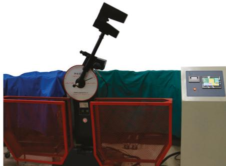
**Figure 2.** Charpy impact testing machine with a hammer having pre-lift angle of 150°.
