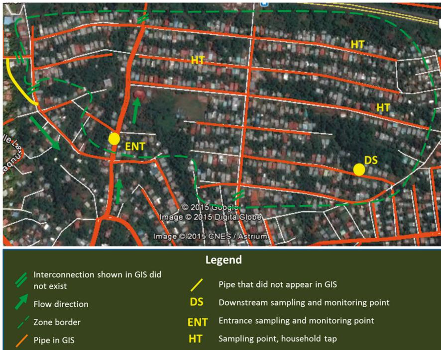
**Figure 2.** Schematic of Study Zone 2. The entrance (ENT) and downstream (DS) locations at which continuous monitoring stations were installed are indicated, as well as the household taps at which water quality grab samples were collected. (Source of satellite images and study zone schematic: Google Earth and IDAAN’s GIS database).
