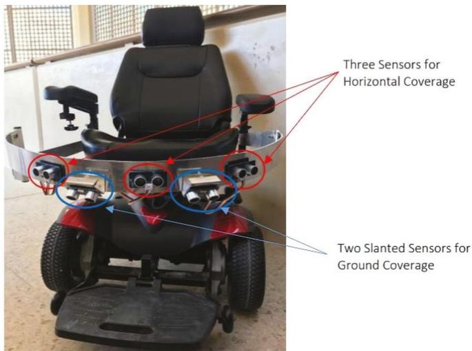
Figure 17. Implemented proximity sensor design.
