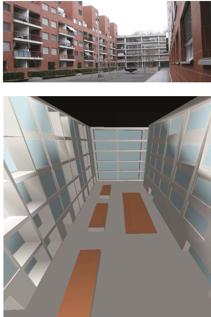
Figure 3. Reference inner yard in original ( above ) and as a simplified geometric model for the ODEON room acoustic simulation ( below ). Absorption coefficient of the materials is coded by their colors, whereby, black stands for the fully absorbing encasing box. Blue and gray represent the reflecting glass or brickwork facade, respectively. The floor is either reflecting smooth unpainted concrete (gray) or absorbing grass (brown).
