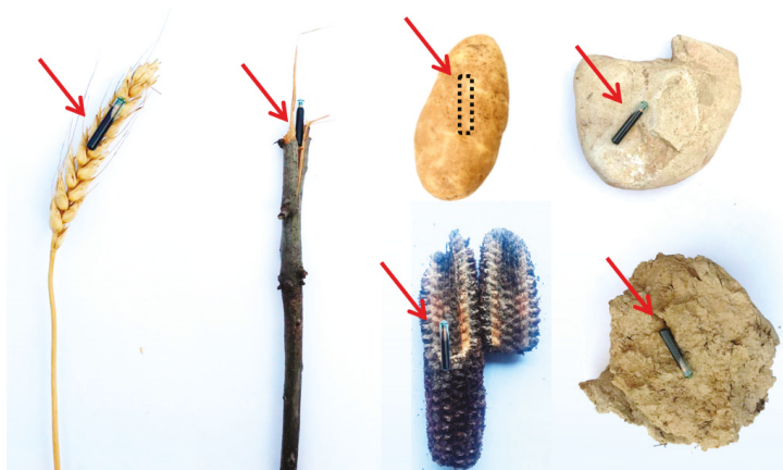
Figure 8. Suggested applications for the use of Radio-Frequency Identification (RFID) to simulate or monitor crop residues, straw, soil clods and potato in agricultural experiments.
