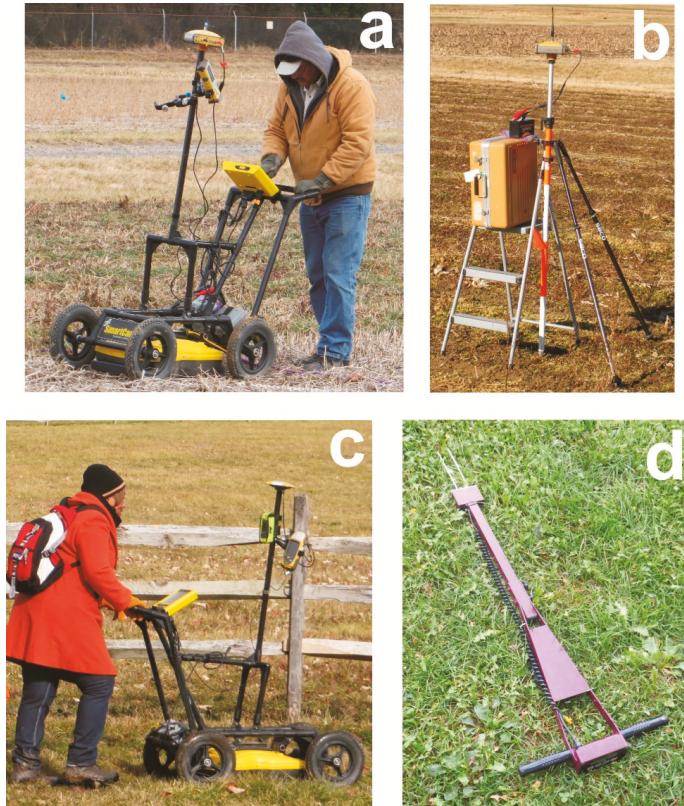
Figure 3. Equipment used in investigation: (a) Noggin GPR system (250 MHz antennas) with GNSS FC-200 rover receiver; (b) GNSS HiPer XT base station receiver; (c) Noggin GPR system (250 MHz antennas) with GNSS GRS-1 rover receiver and PG-S1 hand-held controller; (d) Field Scout TDR-300.
