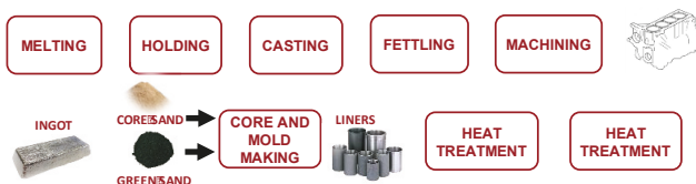
Figure 7. Process flow for Al-alloy engine block manufacturing.
