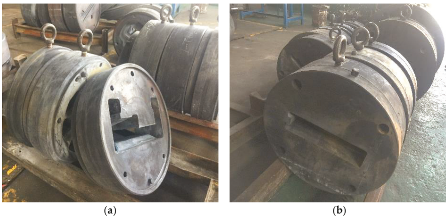
Figure 4. Extrusion dies with customised holes for different aluminium profiles (a) and (b).
