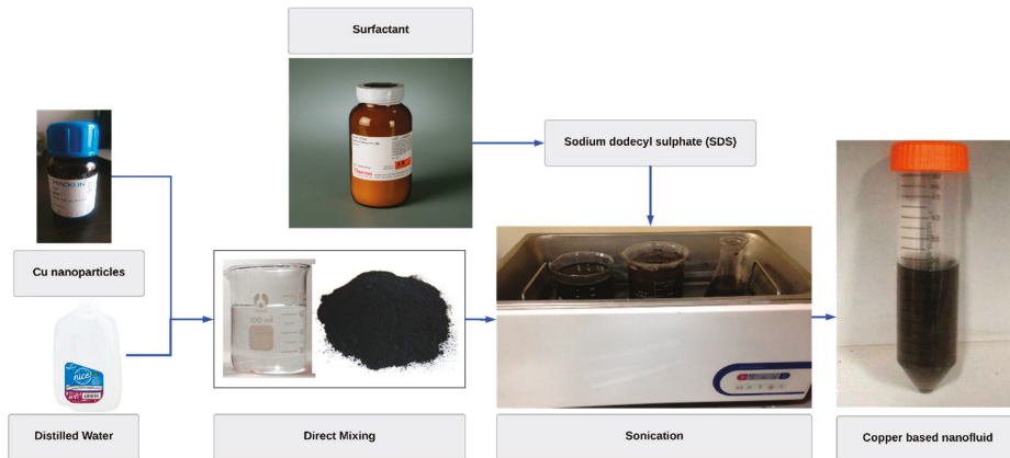
Figure 2. The preparation of copper based nanofluid.
