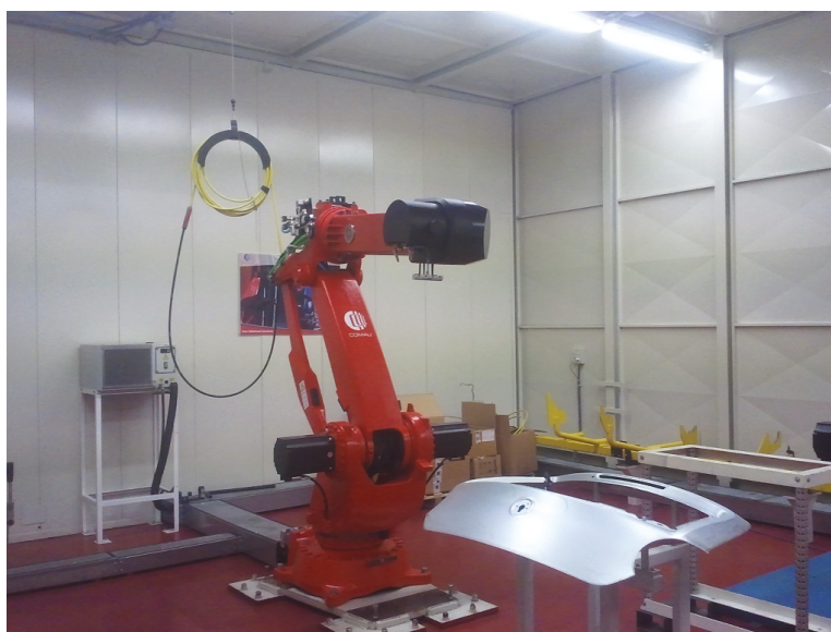
Figure 12. Experimental setting for RLW welding.
