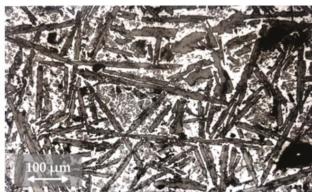
Figure 5. Needles of tricalcium silicate and globular particles of dicalcium silicate in the slag after minute 11 of oxygen blowing, in the melting process B, sample B11.
