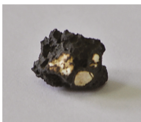
Figure 1. Free lime in the slag at the end of oxygen blowing in the melting process B, sample B27.
