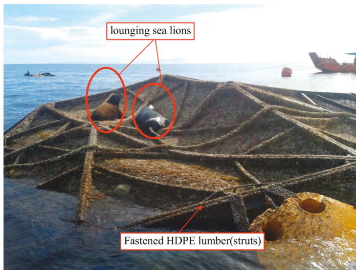
Figure 1. Buckled Aquapod cage made from HDPE lumber and netting (covered with biofouling) with two lounging sea lions on the exposed struts [1].
