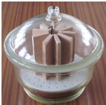
Figure 1. Plywood samples in the glass desiccator.
