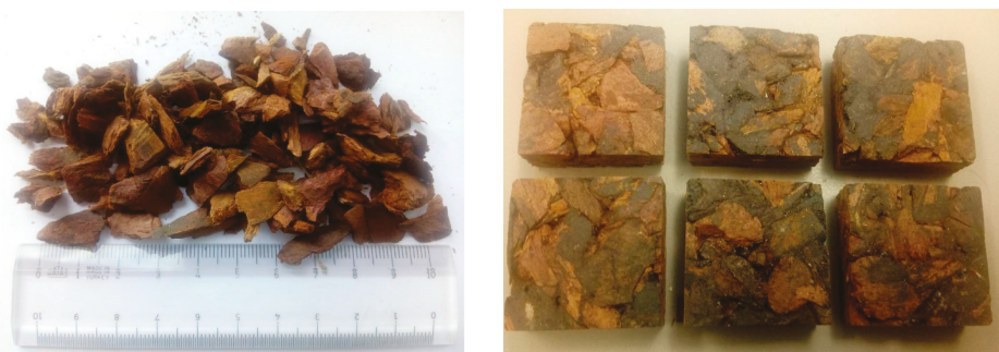
Figure 1. Larch bark particles (8–13 mm) (left) and bark based composite specimens (right) for acoustic measurements.
