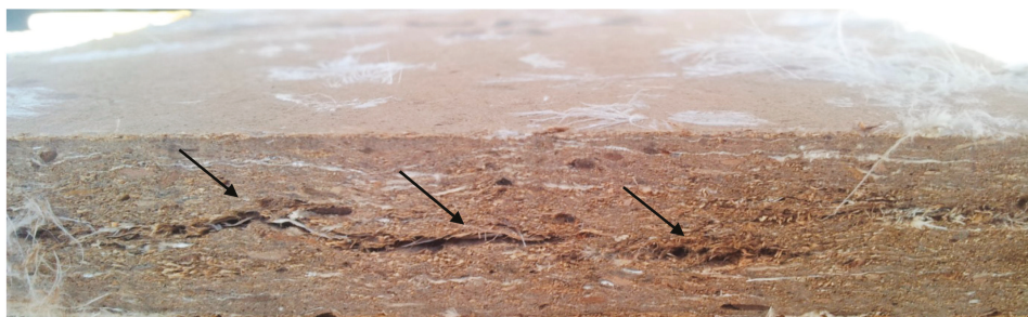
Figure 3. Cracks (blows) (↓) in the core layer of MDF-feather boards (F-10%).
