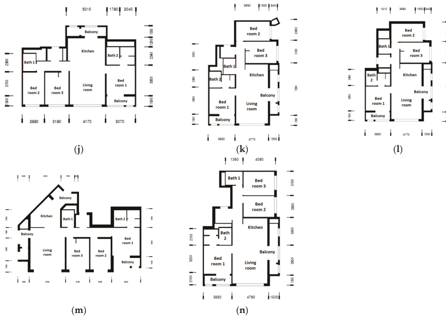
Figure 1. The 14 floor plans of the studied housing units with different floor areas: (a) 33 type; (b) 36 type; (c) 46 type; (d) 59A type; (e) 59B type; (f) 59C type; (g) 74A type; (h) 74B type; (i) 74C type; (j) 84A type; (k) 84B1 type; (l) 84B3 type; (m) 84C type; (n) 84D type.
