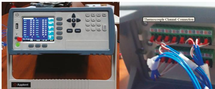
Figure 7. Temperature data acquisition device (T-DAQ).
