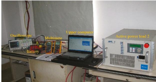
Figure 4. Battery test platform.
