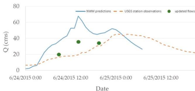
**Figure 5.** River flow at a USGS station at Squaw Creek at Ames. Solid blue line shows the NWM predictions, dashed-red line shows the observations at the USGS station, and green dots show the updated flows.
