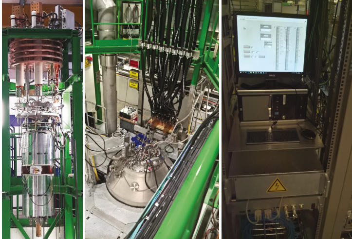
Figure 3. Test facilities of SM18 for testing MQXFS inner triplet quadrupole magnet, including the rack used for the data acquisition and tests (photos provided by E.M.).
