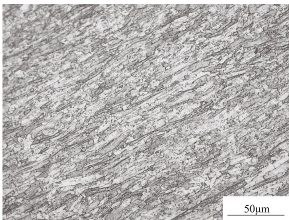
**Figure 1.** The original microstructure of the employed low-carbon ferritic stainless steel.
