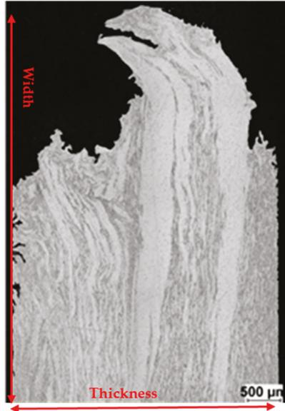
**Figure 3.** Optical micrograph showing a detail of the bar edge with the macroscopic defect. The elongated and work hardened grains at mid thickness appear to be extruded from the microstructure during hot working (2% Nital Etching).
