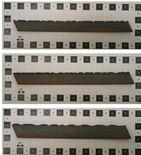
Figure 1. Specimens of flat bar in steel grade 1.4512 affected by jagged borders.
