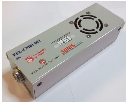
Figure 8. The final developed instrument with external physical dimensions of the aluminum enclosure of 150 mm by 50 mm by 45 mm.
