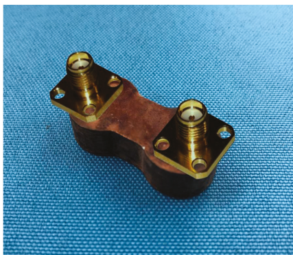
Figure 5. Schematic diagram of mounting position of two SMA connectors on the filter.
