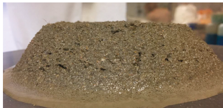
Figure 3. Flow table test for the modified mortar.
