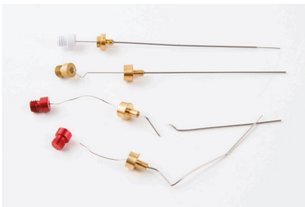
Figure 4. Mechanical failures common to traditional SPME fibers.
