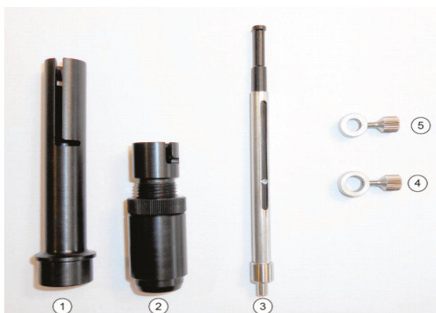
Figure 2. Restek PAL traditional SPME fiber and SPME Arrow manual extraction and injection kit. (1) Extraction guide; (2) injection guide; (3) Arrow/fiber syringe; (4) large inner diameter (ID) locking screw; and (5) small ID locking screw.
