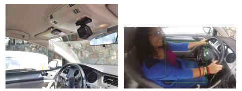
(a) Camera setup (b) Sample daylight Region of Interest (ROI) image. Figure 2. Image acquisition setup.
