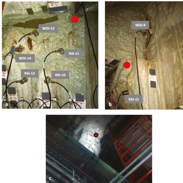
Figure 2. Photographs of the crane maintenance area: (a) Main sensor grid, (b) close-up of sensor on side of column, and (c) view of main grid from the floor level (red dot is at corner).
