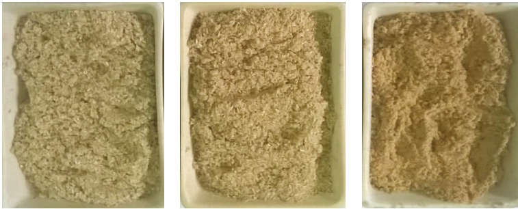
Figure 3. Samples ready for densification: from left to right, the samples of the raw material dried at 60, 100, and 140 °C, respectively, in the dry state are shown.
