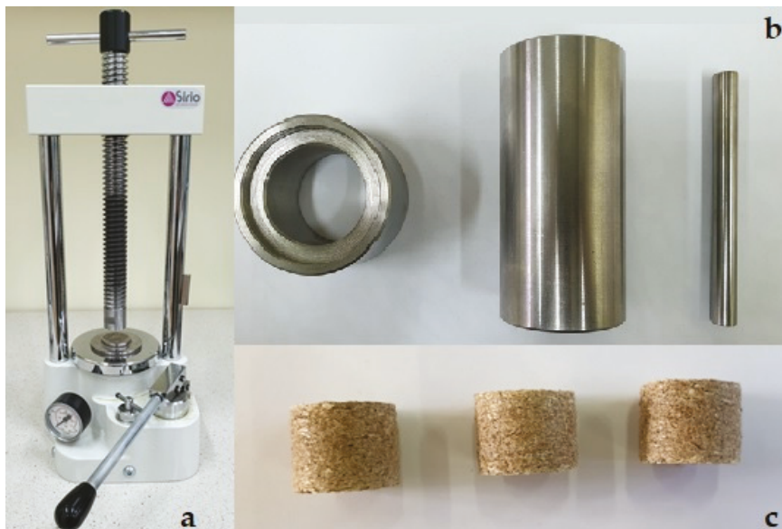
Figure 2. Compaction station: (a) hydraulic press SIRIO P400, (b) compaction chamber and piston, (c) samples.
