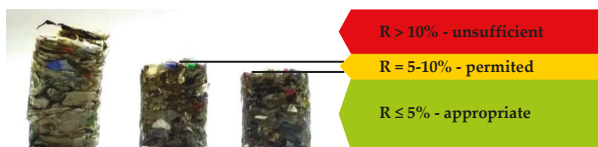
Figure 10. Pellet quality criterion based on the expansion coefficient.
