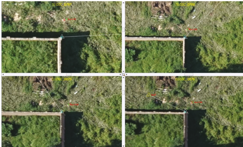
Figure 6. Selection and positioning of the image control points.
