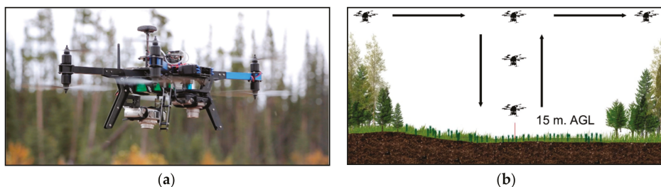
Figure 3. (a) The 3DR X8+ unmanned aerial vehicle (UAV) can collect density samples at a rate of 45 s/ha. (b) The sample-based flight plan used for this study enables a rapid assessment of large forestry blocks. The UAV moves to a sample plot waypoint, descends to a 15 m altitude above ground level (AGL), captures an image, ascends, and continues to the next waypoint.
