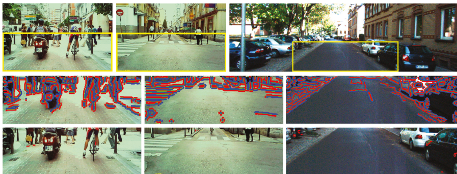
Figure 19. (Row 1) input images; (Row 2) ROI overlaid with brighter (red) and darker (blue) regions across strong edges (green); (Row 3) results of the proposed shadow edge detection method.
