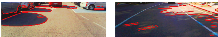
Figure 5. Shadow edge detection obtained by the constraint which relates the red–green and the red–blue proportions of Property 3, i.e., Equation (21).
