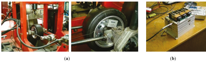
Figure 1. (a) Indoor tire test rig; (b) Acquisition system SoMat2000®.
