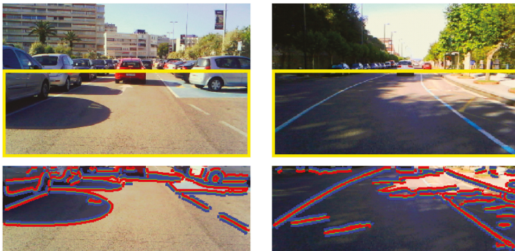
Figure 2. (First row) Bounding box containing the region of interest (ROI) of two input red–green–blue (RGB) images of our dataset. (Second row) Darker (in blue) and brighter (in red) regions on both sides of each edge (in green) of the ROI image.
