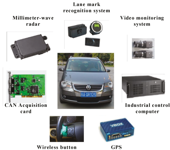
Figure 16. Experimental vehicle used to validate the proposed lane-change decision model in [25].
