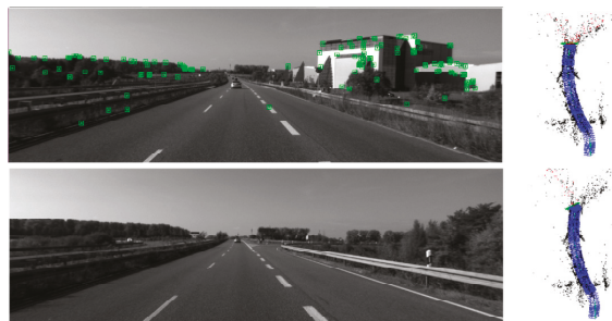
Figure 12. The lost ORB features during tracking on the sequence 01 of KITTI dataset.
