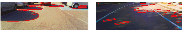
Figure 3. Shadow edge detection of images in Figure 2 obtained using Property 1, i.e., Equation (14).
