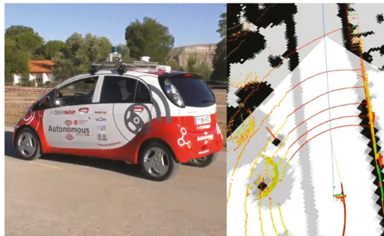
Figure 21. (Left) Autonomous vehicle platform used during the experiments. (Right) Visualization of the LiDAR point cloud (images obtained from [34]).
