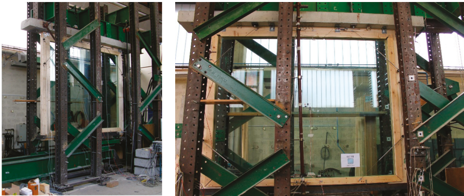
Figure 4. An example of a timber–glass composite system [39,40,88–94].
