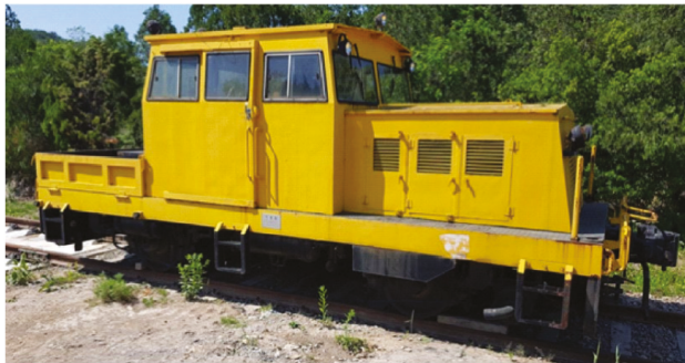
Figure 8. Power car to accelerate the test bogie.
