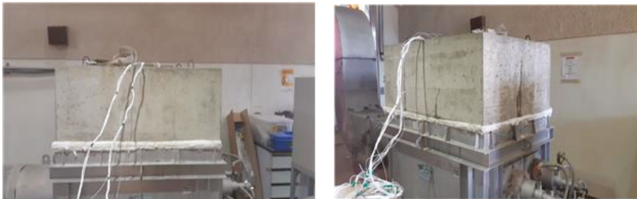
Figure 5. Experimental setup for the fire exposure test using the RABT fire curve.
