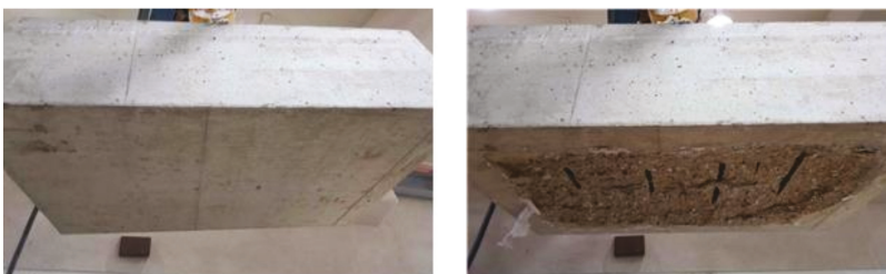
(a) Specimen surface before the fire exposure experiment (b) Specimen surface after the fire exposure experiment
