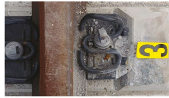
Figure 19. First impact, Case #1: (a) acceleration vs. time (0.3–0.6 s); (b) test bogie at first impact; (c) damage to the hump and rail fastener due to the first impact.
