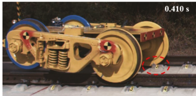
Figure 19. First impact, Case #1: (a) acceleration vs. time (0.3–0.6 s); (b) test bogie at first impact; (c) damage to the hump and rail fastener due to the first impact.
