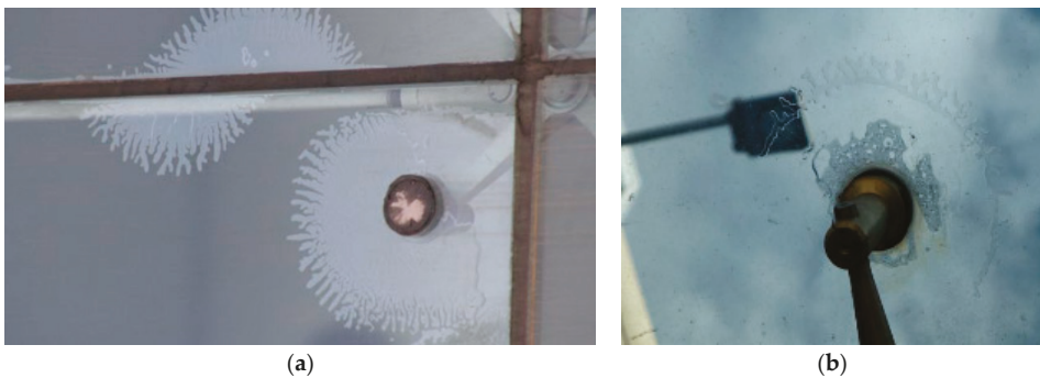
Figure 6. Examples of severe delamination in LG member, in the region of point mechanical restraints. Reproduced with permission from (a) [36] and (b) [37].
