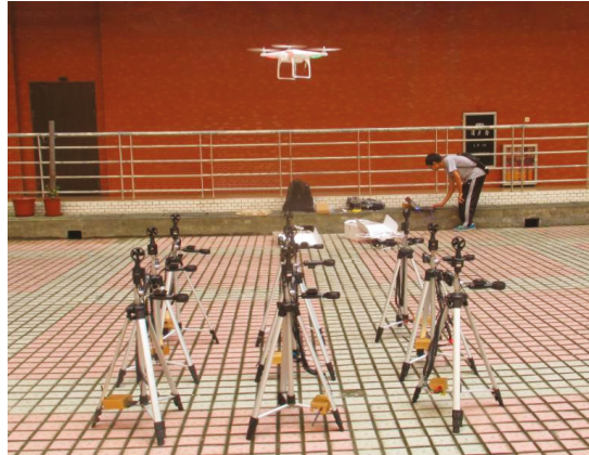
Figure 6. Actual test of downwash flow field.
