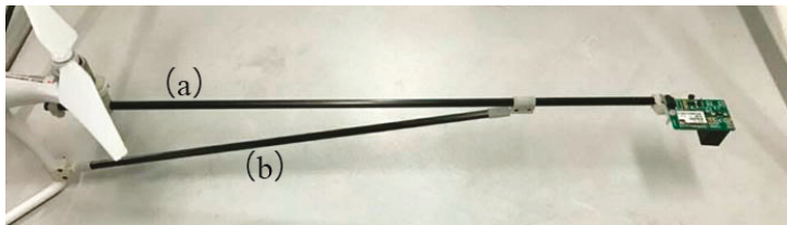
Figure 8. Design of UAV support and damping rod. (a) Support; (b) damping rod.
