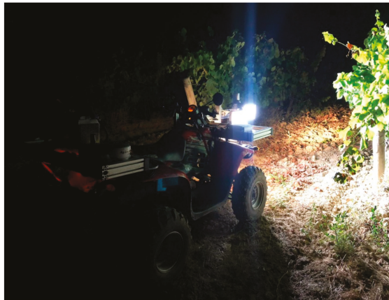
Figure 1. Mobile sensing platform for on-the-go image acquisition: a modified all-terrain vehicle (ATV) incorporating a red, green, blue (RGB) camera, Global Positioning System (GPS), and an artificial illumination system mounted on an adaptable structure.
