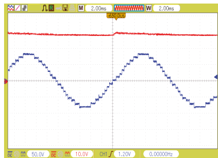
Figure 17. The voltage of V_{C2} experimental results.
