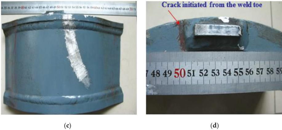
**Figure 1.** The crack position and the Macro morphology of the crack: (a) the crack position found in site; (b) the model of bogie frame and the positioning block; (c) and (d) the macro pictures of crack initiated from the weld toe of positioning block.
