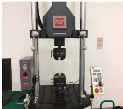
**Figure 2.** MTS (Systems Corporation) fatigue tensile testing machine.
