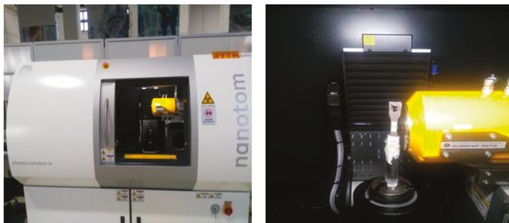
Figure 4. X-ray micro-computed tomography system.
