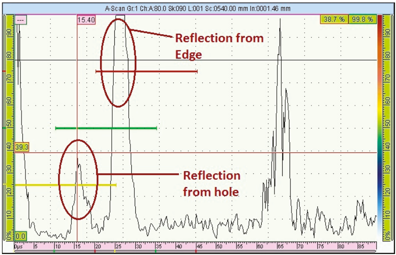
Figure 11. Typical PAUT guided wave signal of flaw detection for CFRP sample.
