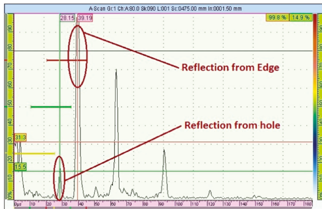
Figure 10. Typical PAUT guided wave signal of flaw detection for (a) Al-1 sample and (b) Al-2 sample.
