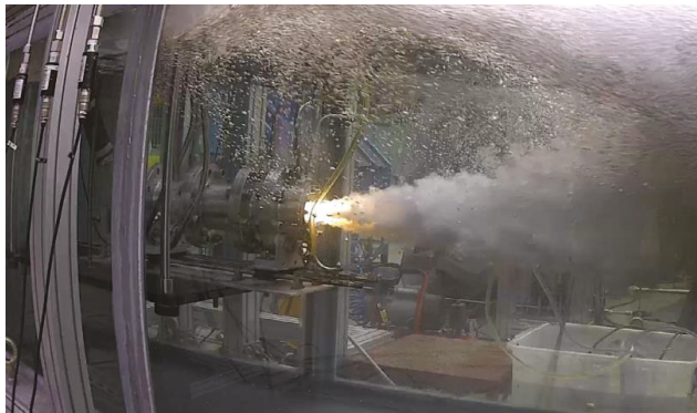
Figure 14. Snapshot of underwater hot-firing test.
