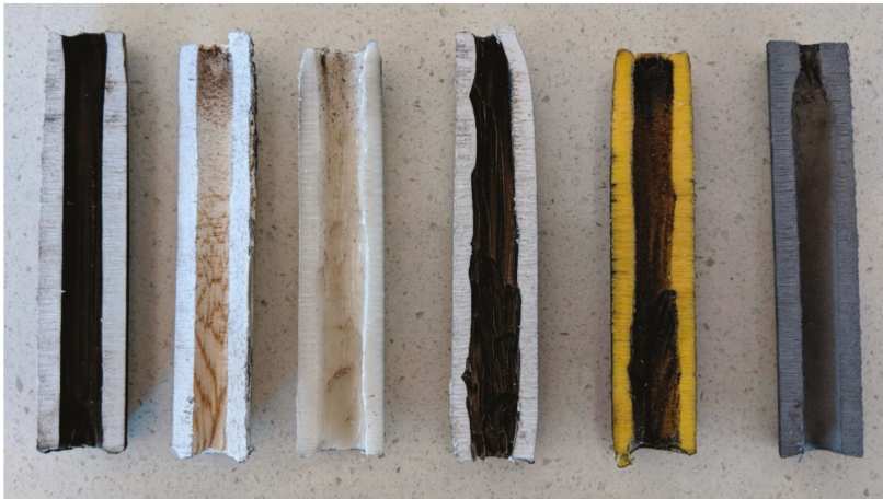
Figure 5. Cross section of each different small-scale fuel grain, left to right: ABS, PLA, PP, ASA, PTEG, and AL.
