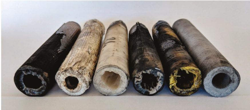
Figure 4. Combustion port comparisons, left to right: ABS, PLA, PP, ASA, PTEG, and AL.
