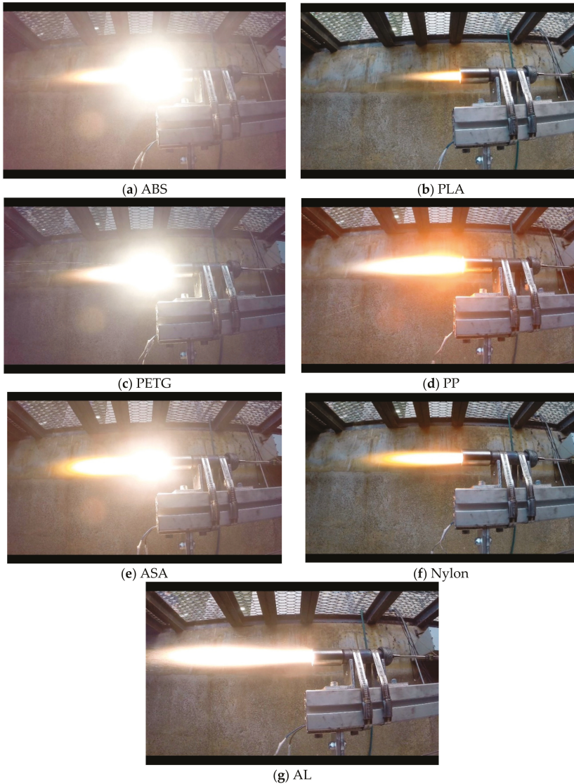
Figure 3. Small-scale testing of fuel grains 3D-printed from different fused deposition manufacturing (FDM) materials.
