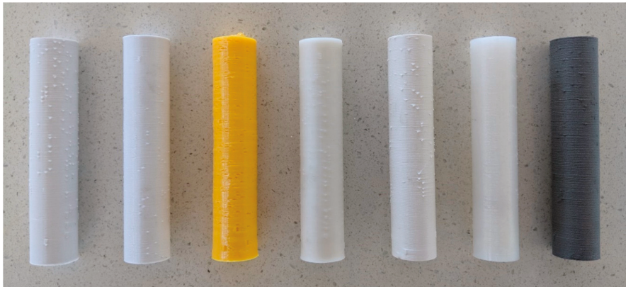
Figure 2. Small-scale fuel grains, left to right: ABS, PLA, PETG (Polyethylene terephthalate glycol), PP, ASA, Nylon, and AL (PLA with aluminum particles).
