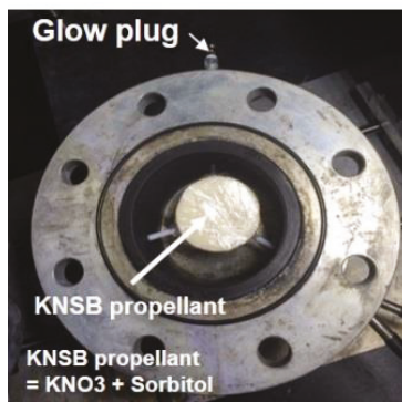
Figure 9. KNSB igniter mounted in pre-chamber.
