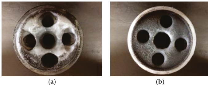
Figure 7. Fuel grain after combustion, (a) front view; (b) rear view.
