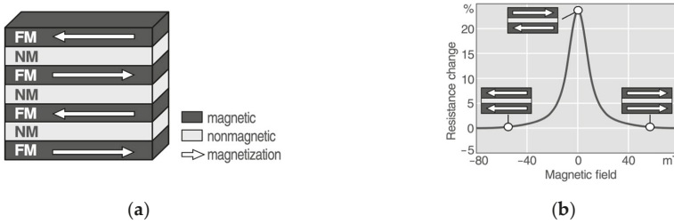
Figure 10. GMR sensor principle. (a) GMR multilayer structure with FerroMagnetic (FM) and Non FerroMagnetic (NM) layers; (b) Resistance characteristic according to an applied magnetic field, reproduced from [9]. Copyright 2007, Robert Bosch GmbH.
