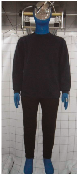
Figure 5. Evaluation of the clo level using a manikin with winter clothing.
