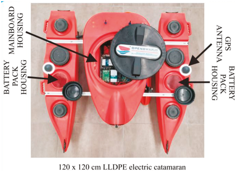
Figure 3. Photo and technical details of the latest OpenSWAP vehicle.
