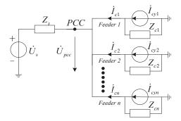
Figure 3. Equivalent circuit of the power system with concentrated multiple harmonic feeders.
