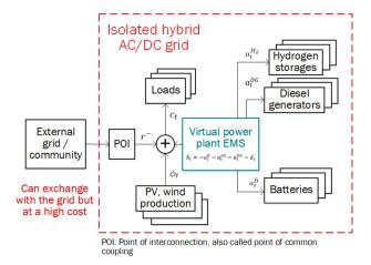
**Figure 3.** A general scheme of the hybrid AC/DC power grid featuring distributed energy resources (DERs) associated with possible inclusions options batteries, hydrogen storages and diesel unit devices.
