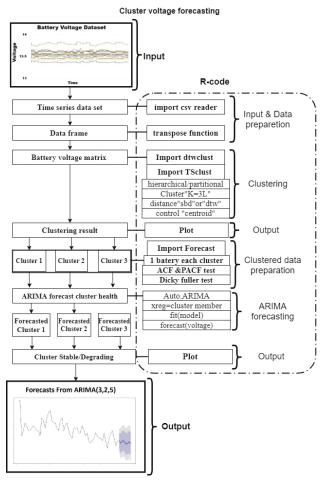
Figure 3. Battery cluster inconsistency and battery degradation forecast method.
