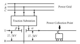
Figure 1. Train-network coupling system.
