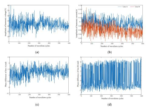
**Figure 13.** (a) Harmonic voltage data at PCC point; (b) Harmonic current data of each feeder; (c) Phase difference data between harmonic voltage and harmonic current of Line A; (d) Phase difference data between harmonic voltage and harmonic current of Line B.
