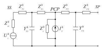
Figure 2. The equivalent circuit of train-network coupling system.
