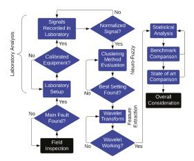
Figure 4. Method flowchart for insulator withdrawal and model evaluation.
