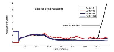
**Figure 16.** One-year actual resistance value, resistance rise in Battery 6, as well as Stable Resistance for Battery 15, 19, and 36, validate the proposed method.
