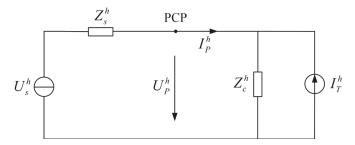
Figure 3. Thevenin equivalent circuit.
