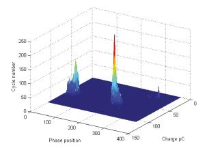
Figure 14. Failure in S-phase cable termination.
