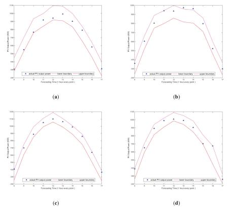
**Figure 9.** Interval forecasting results of four days for a PV power plant. (a) 6 August 2011; (b) 30 October 2011; (c) 14 March 2012 and (d) 19 May 2012.
