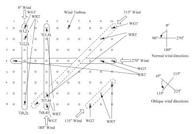
**Figure 4.** Normal and oblique wind delivery in the Horns Rev OWF, Denmark. Note, WGT is the wind energy-giving turbine, and WRT is the wind energy-receiving turbine.
