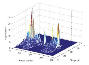
Figure 16. Failure in T-phase cable termination.
