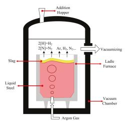
Figure 1. Schematic representation of a VTD.
