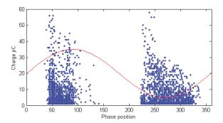
Figure 11. Typical 2D partial discharges (PD) pattern.
