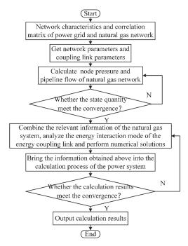
Figure 1. Flow chart of EGIES flow calculation.
