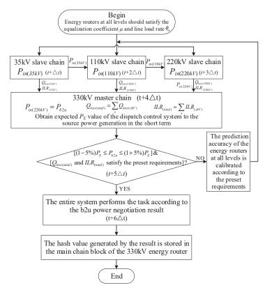
Figure 4. Blockchain-based transmission and distribution network consultation mechanism.
