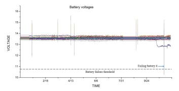
Figure 4. One year battery voltages in data center.
