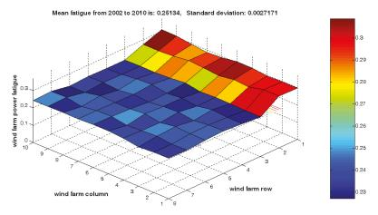
Figure 8. Conventional farm fatigue distribution (2002–2010, Horns Rev OWF, Denmark).
