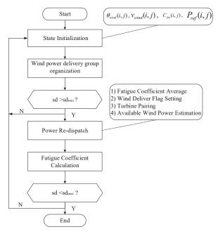
Figure 6. Workflow of the wind farm main controller.
