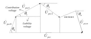
Figure 4. Phasor projection diagram of the harmonic voltages.
