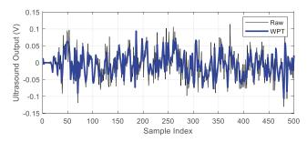
Figure 2. Comparison between original and rebuild signal using Wavelet Packets Transform (WPT).
