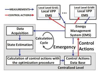
Figure 4. Hybrid network emergency control calculation cycle.
