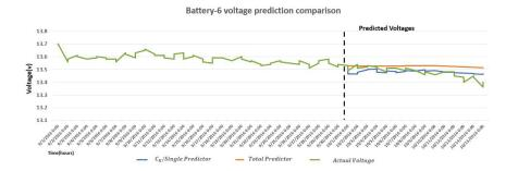
**Figure 11.** Comparison of measured and ARIMA forecasted voltage with Clustered (Single) predictor of Battery 6.
