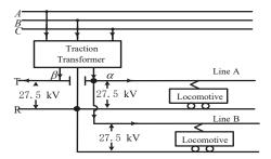
Figure 12. Schematic diagram of the "traction net-locomotive" system.
