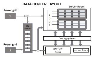
Figure 1. Data center layout. PDUS = Power Distribution Units.
