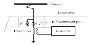
Figure 8. Schematic diagram of measurement.
