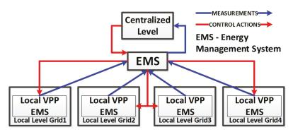
Figure 2. Two-level operational management system.
