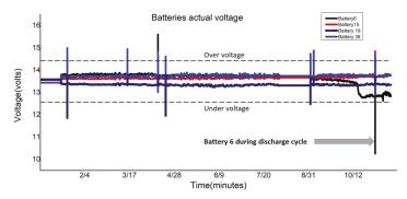
**Figure 15.** One-year actual voltage value, voltage drop in Battery 6, as well as stable voltages for Battery 15, 19, and 36, validate the proposed method.
