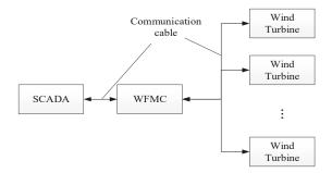
Figure 2. The power control and communication scheme in an OWF.
