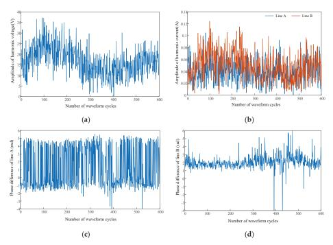
**Figure 14.** (a) Harmonic voltage data at PCC point; (b) Harmonic current data of each line; (c) Phase difference data between harmonic voltage and harmonic current of Line A; (d) Phase difference data between harmonic voltage and harmonic current of Line B.
