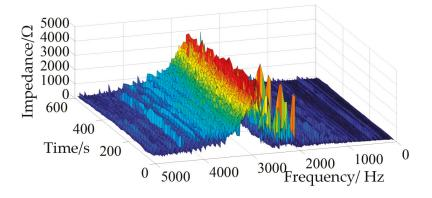
(a) Amplitude of the harmonic impedance with measured data.
