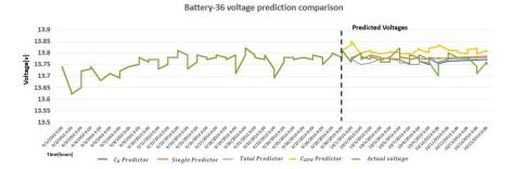
**Figure 14.** Comparison of measured and ARIMA forecasted voltage with  $C_K$ , Single, Total, and  $C_{DTW}$  predictor of Battery 36.
