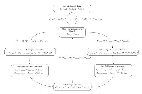
Figure 5. Improved control topology of the wind farm main controller.
