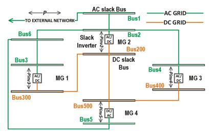
Figure 10. The hybrid AC/DC test system.
