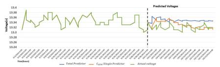
Figure 13. Comparison of measured and ARIMA forecasted voltage with Total predictor of Battery 19.
