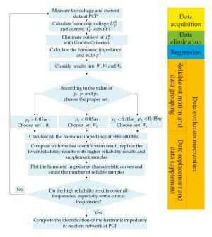
Figure 4. The flowchart of harmonic impedance identification.
