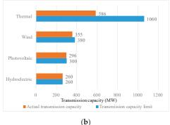
Figure 5. (a) Simulation results of the optimal scheme of the actual output of each energy plant; (b) the optimal output scheme for each power plant when the power demand is 2000 (MW).
