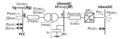
Figure 5. Steady state VSC station model.
