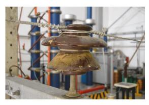
Figure 1. Contaminated insulator removed from a 25 kV rural area distribution system.
