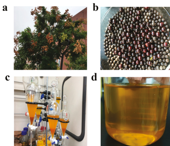
Figure 2. (a) Koelreuteria paniculata plant (KP) (b) KP seed (c) Transesterification (the process of optimization) (d) Pure KP biodiesel after processing.
