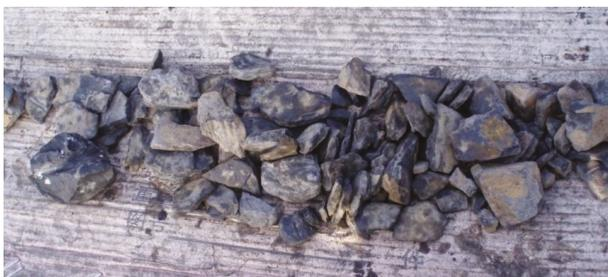
Figure 8. Core samples obtained from the collapse column.
