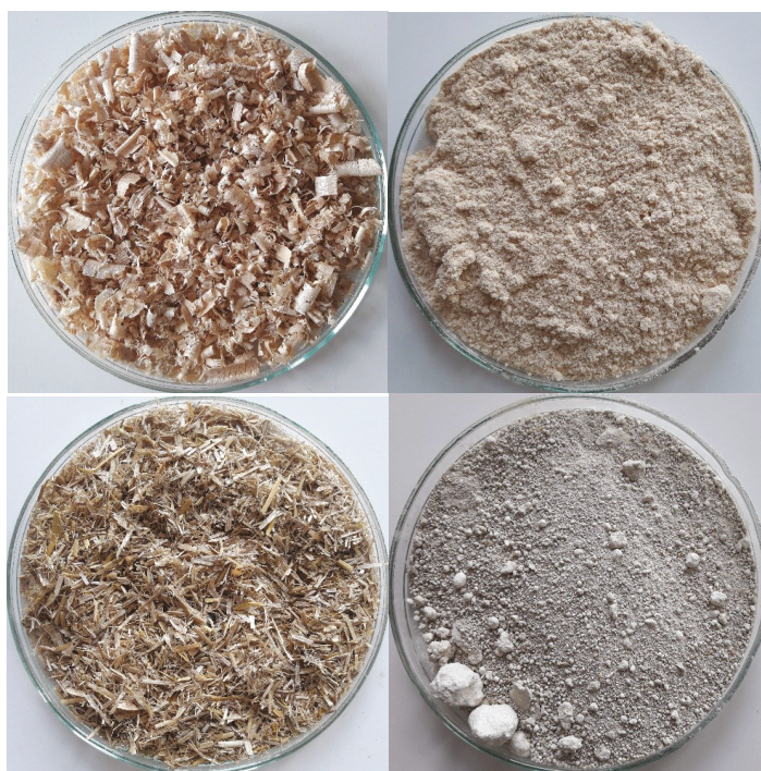
Figure 1. Input materials used in the study—wood shavings, wood dust, straw and limed sewage sludge.
