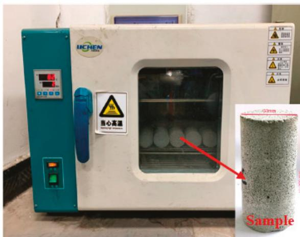
Figure 2. Constant temperature vacuum drying oven.
