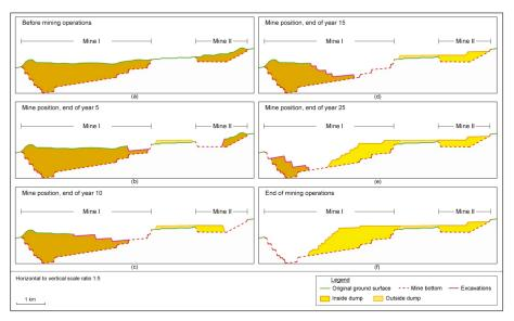
Figure 4. Sequence of mine development in the cross section A-A' of Figure 2.
