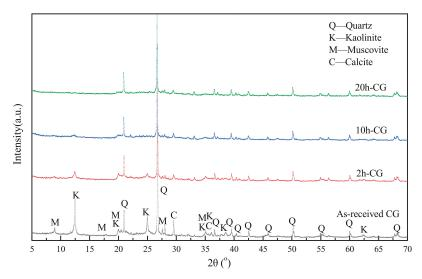
Figure 3. XRD spectra of as-received coal gangue and mechanical activation coal gangue.
