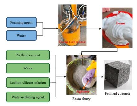
Figure 1. Procedure of specimen perpetration.
