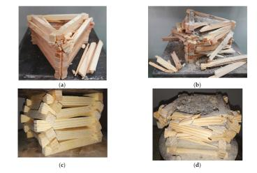
Figure 8. Wooden cribs models after compression test: (a) Three-point; (b) Three-point filled with gangue; (c) Four-point; (d) Four-point filled with gangue.
