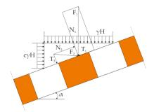
Figure 12. Scheme of loading of cribs in an inclined orebody.
