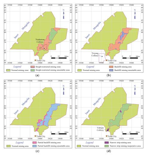
**Figure 18.** Applicability partition of water conservation coal mining method (Xi'an geodetic coordinate system 1980; in km): (a) Height-restricted mining application area; (b) Backfill mining application area; (c) Partial backfill mining application area; (d) Narrow strip mining application area.
