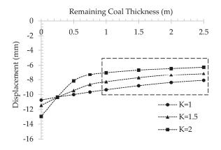
Figure 10. Correlation between roof displacements and RCT.
