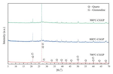
Figure 8. XRD spectra of CGGP specimens.
