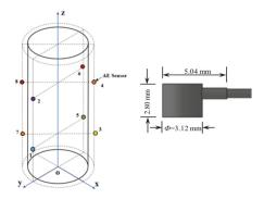
Figure 3. Distributions and dimensions of an AE sensor.
