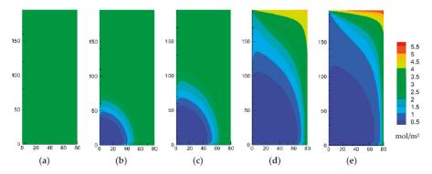
**Figure 10.** Concentration distribution in gas evacuation process: (a) t = 0 day; (b) t = 0.5 day; (c) t = 1 day; (d) t = 3 days; (e) t = 5 days.
