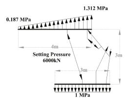
Figure 7. Pressure distribution for modeling shield support.
