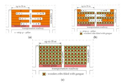
**Figure 11.** Strip mining method with the three stages of exploitation in relation to the management of wooden cribs filled with gangue: (**a**) First stage; (**b**) Second stage; (**c**) Third stage.
