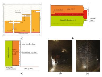
**Figure 3.** Strip mining method in Olkusz-Pomorzany mine: (a) Unidirectional and bidirectional exploitation; (b) Exploitation with a barrier pillar; (c) Exploitation without a barrier pillar; (d) Construction of wooden dam with backfilling pipeline; (e) Additional wooden support in a room.
