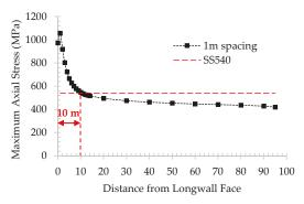
Figure 18. Maximum support axial stress along the gate-entry for 100 m of depth.
