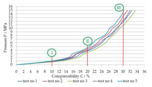
Figure 5. Pressure–compressibility characteristics of gangue (dolomitic limestone): I, II, III—10%, 20%, and 30% of compressibility, respectively.
