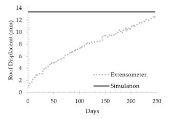
Figure 9. Comparison between extensometer results and simulation results.
