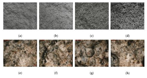
**Figure 6.** Pore structures of different foam content in 1 kg mass of solid powder: (**a**) 0.5 L foam; (**b**) 1.0 L foam; (**c**) 1.5 L foam; (**d**) 2.0 L foam; (**e**) 0.5 L foam (×500 times); (**f**) 1.0 L foam (×500 times); (**g**) 1.5 L foam (×500 times); (**h**) 2.0 L foam (×500 times).
