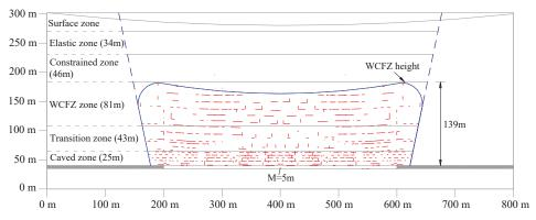
Figure 13. WCFZ of 5 m mining height of sand-soil-bedrock stratigraphic structure.
