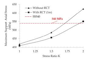
Figure 12. Maximum support axial stress for 100 m of depth (1 m spacing).
