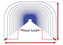
Figure 4. Modelling of steel arch for roof support.
