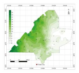
**Figure 17.** Maximum (theoretical) allowable mining height contour. (Xi'an geodetic coordinate system 1980; in km).
