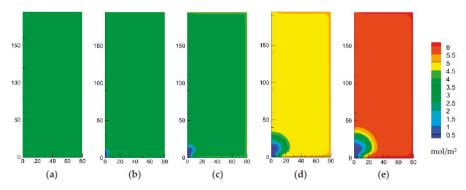
**Figure 11.** Concentration distribution in gas sealing process: (a) t = 0 day; (b) t = 0.5 day; (c) t = 2 days; (d) t = 4 days; (e) t = 6 days.
