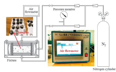
Figure 3. Gas permeability measurement system.
