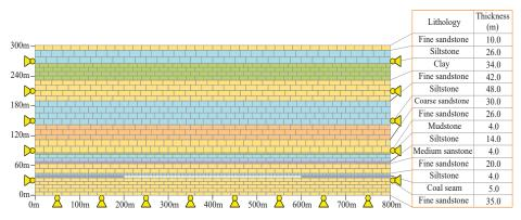
Figure 12. Numerical simulation model of sand-soil-bedrock stratigraphic structure.
