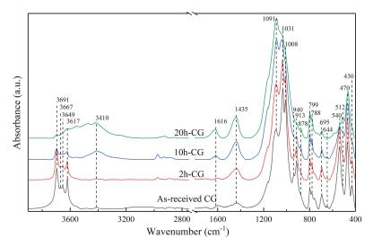
Figure 4. FTIR spectra of as-received coal gangue and mechanically activated coal gangue.
