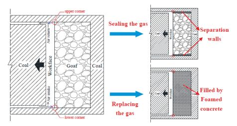
Figure 8. Schematic diagram of application modes.
