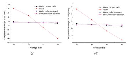
**Figure 5.** Average level of indicators under different factors: (**a**) average level of dry density; (**b**) average level of gas permeability; (**c**) average level of compressive strength of the 3rd day foamed concrete; (**d**) average level of compressive strength of the 28th day foamed concrete.
