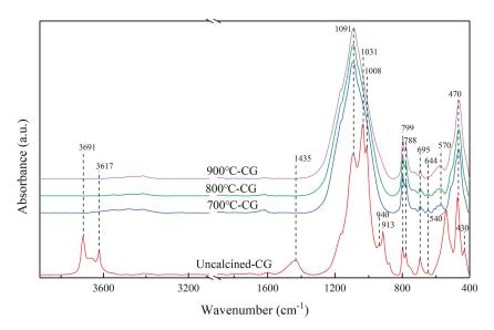
Figure 6. FTIR spectra of thermally activated coal gangue and uncalcined-CG.
