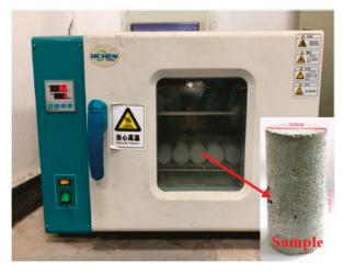
Figure 2. Constant temperature vacuum drying oven.
